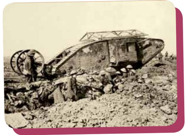
*Mark 1 tank of C Company with anti bomb roof
